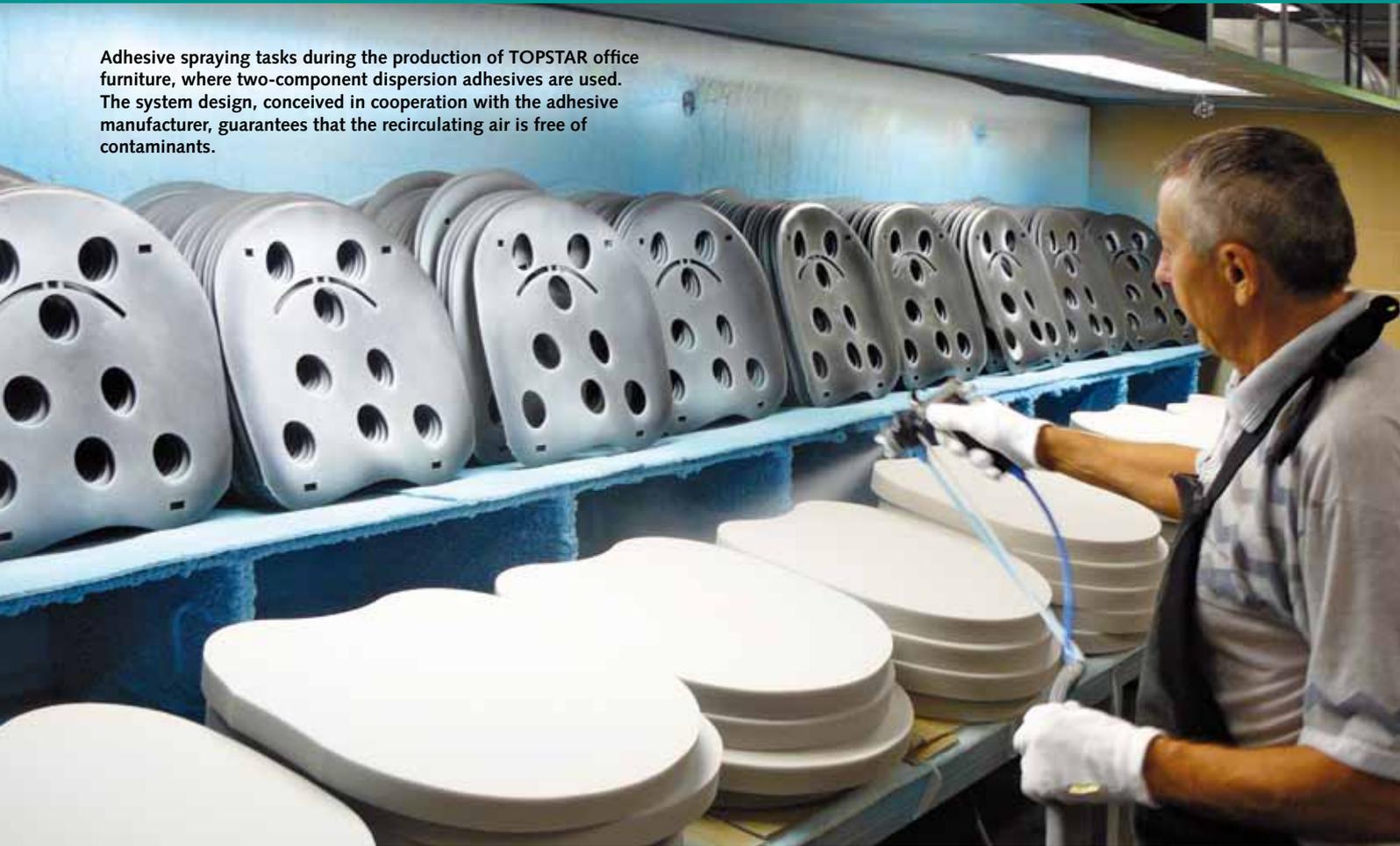
At TOPSTAR GmbH in Langenneufnach near Augsburg, Germany, four large and sixteen small adhesive spray booths have been installed to take care of specific operations. WALTHER PILOT also supplied special spray guns with double nozzles for use with two-component dispersion adhesives. The conversion to water-based media created a need for new, high-power filtration units with total capacities of 35,000 m<sup>3</sup>/h.
