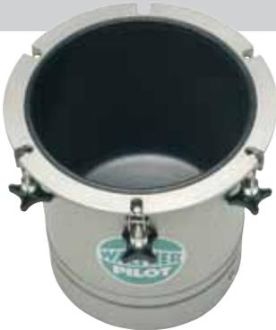
Inliners lie like a skin on the pressure tank's inside surface and effectively protect it from contamination. As soon as the inliner reaches the maximum degree of soiling it can be easily replaced with a new one. This eliminates any need for cleaning agents and for costly, labor-intensive tank cleaning work. Only the pipe to the material outlet, the agitator shaft and the impeller elements need to be cleaned.
