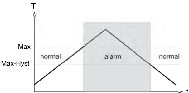
The change to the alarm state is indicated by the integrated red LED and a cleartext in the display. While in the normal state the switching outputs are at the level of the supply voltage; in the alarm state they are at 0 V, so that a wire break would also display as an alarm state at the signal receiver. Overload of the switching output is detected, indicated on the
