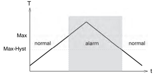
A switchover delay time ( $t_{DS}$ ) can be applied to the switchover to the alarm state. Equally, one switch-back delay time ( $t_{DR}$ ) of several can be applied to switching back to the normal state.
