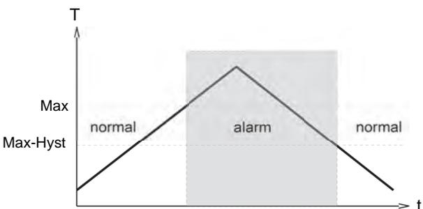
The change to the alarm state is indicated by the integrated red LED and a cleartext in the display. While in the normal state the switching outputs are at the level of the supply voltage; in the alarm state they are at 0 V, so that a wire break would also display as an alarm state at the signal receiver. Overload of the switching output is detected, indicated on the display ("Check S1 / S2"), and the switching output is switched off.
