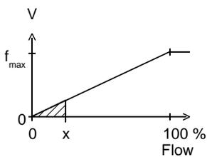
f<sub>max</sub> selectable in the range of up to 2000 Hz
