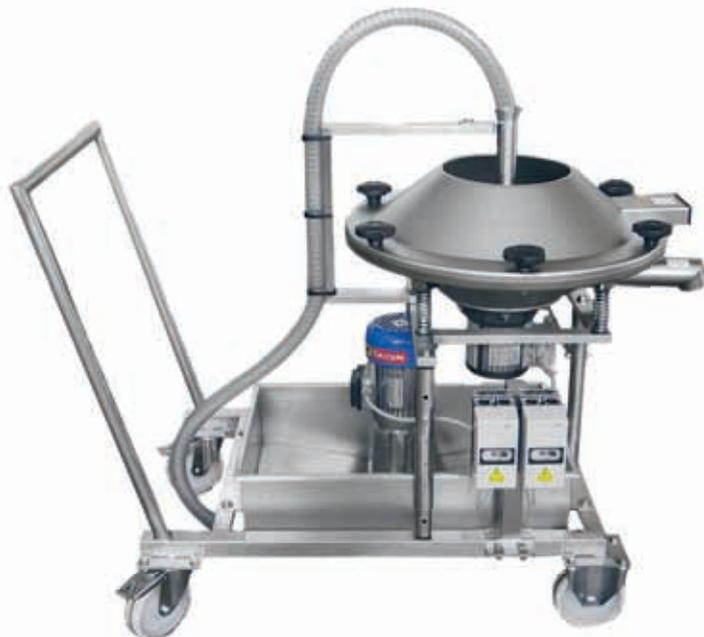
Iron removal filter operating by pressure, with permanent magnets. The compact dimensions, high magnetic force of the neodymium bars and the water-tight enclosure make this system ideal for use within glazing lines, both on tanks and along glaze transfer pipes.
