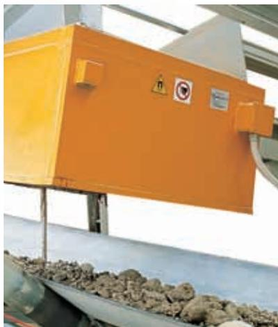
Electromagnetic iron remover with plates for powder and raw materials of established particle sizes, featuring automatic cleaning system, especially designed for installation on mill feeding belts.
