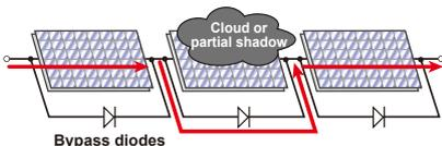
When a solar panel is obscured by a partial shadow (or when it fails), the current bypasses the panel in order prevent any drop-off in generating efficiency.
