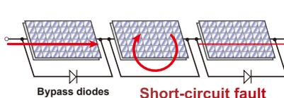
When a short-circuit fault occurs, the generated current flows in a loop, making it impossible to capture the generated power, resulting in lowered efficiency.
