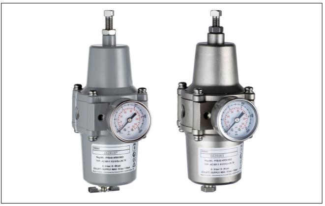
Control of instrument supply air pressure, and removal by filtration of dust particles and water content. FRS02 and FRS03 are dedicated for direct mounting to valve positioners SRI990, SRD998 SRD991, and SRD960.
