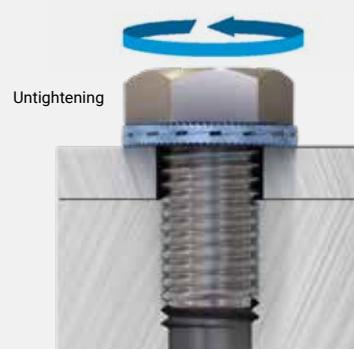
When the fastener is untightened, sliding will occur between the two washers. The upper washer is locked to the nut or bolt head by the serrations. The lower washer does not rotate as its serrations are locked into the surface being clamped.
