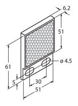
Rectangular reflector, reflection coefficient 2.0, material acrylic, ambient temperature -20 ... +60 °C, microprism geometry
