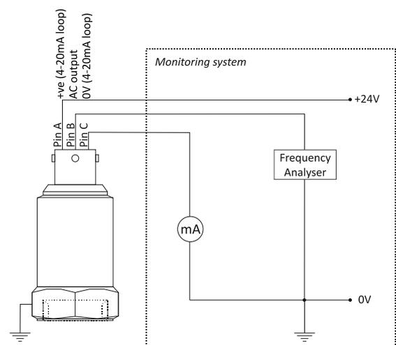
To avoid spurious signals, the body of the sensor must be grounded by the machine or by a grounded connector shell. The monitoring system 0V should also be grounded.
