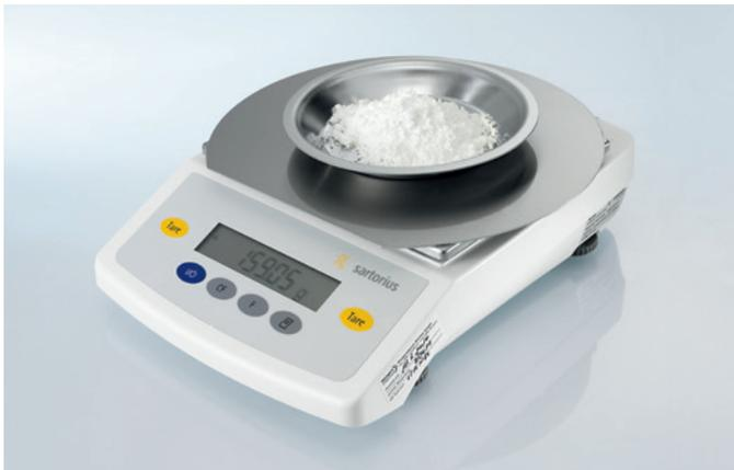
Compatible high-precision laboratory balance to 810 g with weighing pan that is ideally suited to all test sieves up to ø 220 mm
