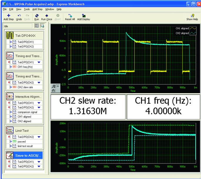
NI LabVIEW SignalExpress™ Tektronix Edition is a fully interactive measurement acquisition and analysis software developed jointly with National Instruments and optimized for the MSO/DPO Series.
