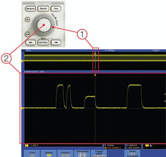
Wave Inspector controls provide unprecedented efficiency in viewing, navigating, and analyzing waveform data. Zip through your 10M point record by turning the outer pan control (1). Get from the beginning to end in seconds. See something of interest and want to see more details? Just turn the inner zoom control (2).
