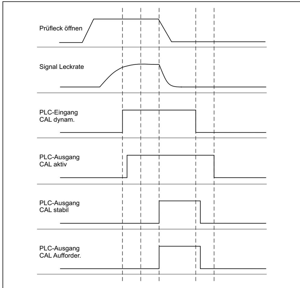
Fig. 7 External dynamic calibration with IO1000 using the example of sniffer line SL3000XL, description of PLC inputs and outputs: See page 48
