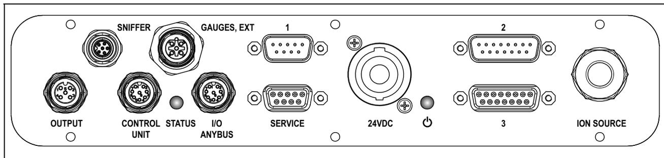
Fig. 3 MSB box connections
