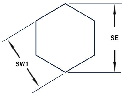
SW: Rivet nut exterior measurement flat side to flat side.
