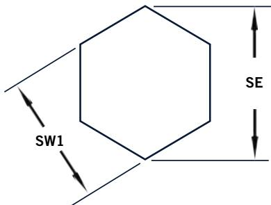
SW: Rivet nut exterior measurement flat side to flat side.
