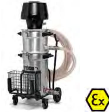
Air powered ejector vacuum cleaners have no moving parts, motors or pumps. They do not require electricity and provide enormous advantages for demanding operations in industry, shipping and offshore. They are used to collect any industrial product or material (liquids, dusts or granules) that can be conveyed along a suction hose.
