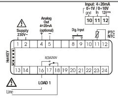
Probe: Pt100=11 - 10 (12); Thermocouple J, K, S= 11(+) - 10(-) 115Vac supply: 1-2; 24Vac supply: 1-2
