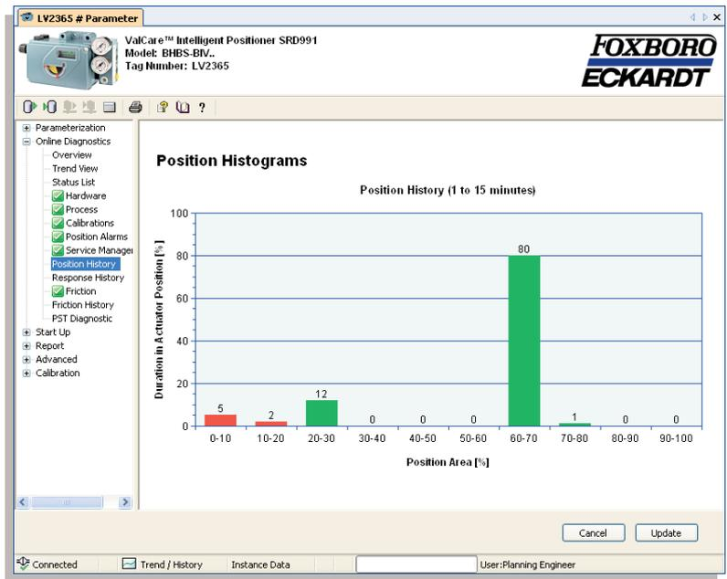
time. The Stem Friction histogram is an additional tool that can be used to identify valve stickiness which is a common valve problem.
