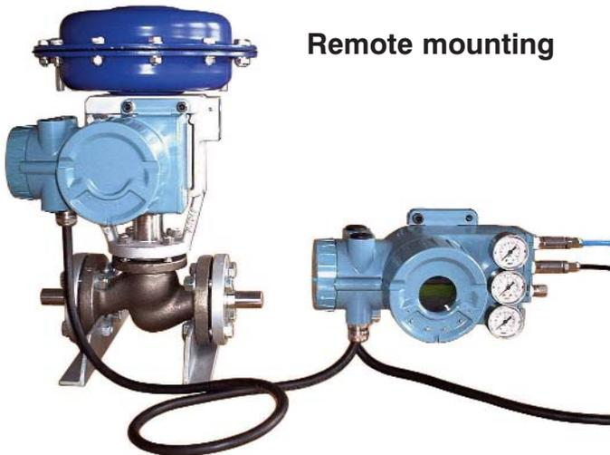
This remote application is used in applications where high temperatures or vibration are present and can result in negative influences to the control. It can also be used in places that are not easy to reach, to ensure an easier handling of the unit, or for a cylinder with large stroke.
