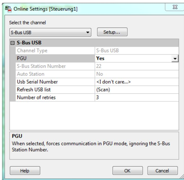
The activation of the PGU option ensures that the PCD3.Mxxxx connected directly to the PC can be communicated independently of the configured S-Bus address.
