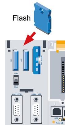
To enable use on a PCD3.M3xx0, the memory modules PCD3.Rxxx are available, which contain a PCD7.Rxxx and can be plugged into an I/O slot (0 ... 3) of a PCD3 CPU.
