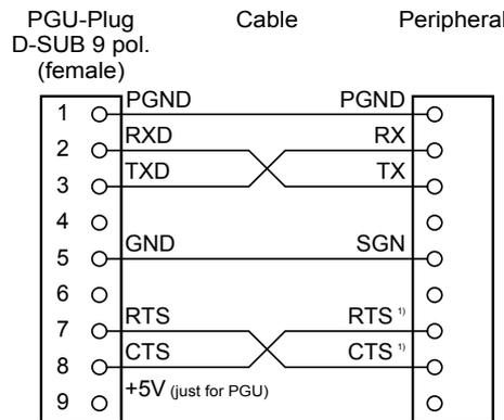
1) When communicating with terminals, check whether certain connections are to be bridged or to be set by the command SOCL on 1 or 0. Generally the use of handshake (RTS / CTS) is recommended (see also manual 26/795, series PCD7. D23x, graphics terminals).
