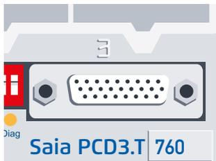
This connector can be used to add up to 3 LIO module carriers to the RIO (with PCD3.K010 connector). This way, 256 I/Os can be realized per RIO.
