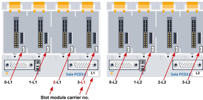
All PCD3 module carriers and the extension cable PCD3.K106 / 116 are accompanied by a matching set of labels as an additional option for labeling.
