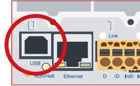
When a PCD3.Mxxxx is connected to a PC for the first time via the USB interface, the operating system of the PC automatically installs the relevant USB driver.
