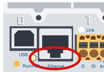
Ethernet connection without LEDs
