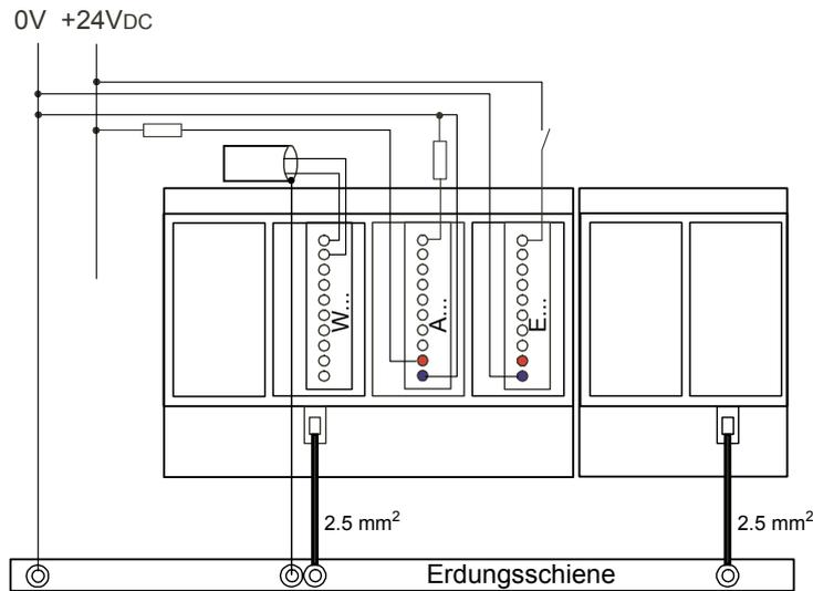
The lower part of the PCD3 module housing contains a shielding and grounding plate. Combined with the shielding and earthing plate in the module carrier, this forms the common, large-area user mass for all I/O modules and the external power supply.
