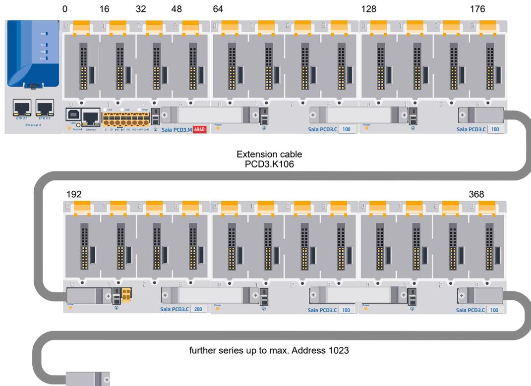
The address of the first module in a second or third series is determined by the address of the last module in the previous series +16.
