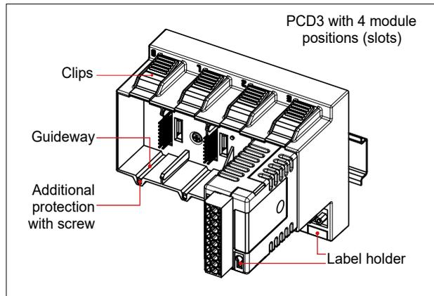
Labeling of the module carriers and I/O plug-in modules
