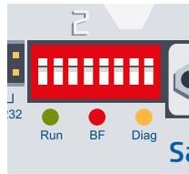
The Profibus address is set to binary on the PCD3.T76x by means of a DIP switch.
