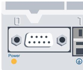
The bus is designed for a baud rate of up to 1.5 Mbps. More detailed specifications of the Profibus communication can be found in the manual 26/765, Profibus DP.
