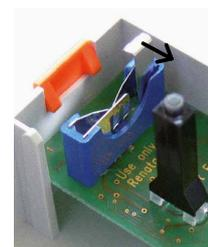
1) Replacing the battery with the Saia PCD® off does not result in program/data loss as long as the Saia PCD® Supercap has not been depleted.
