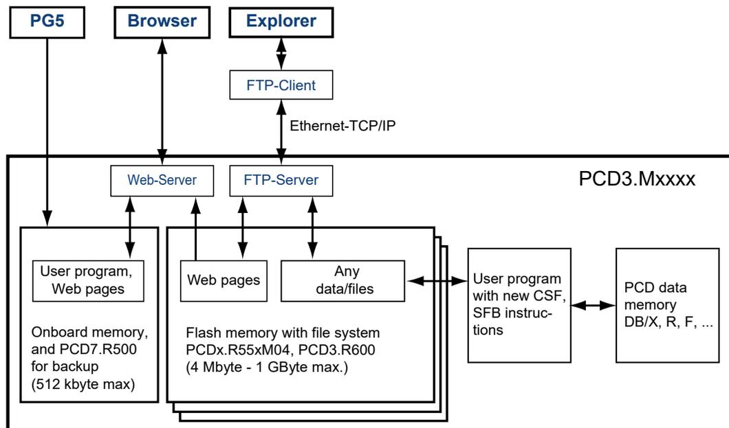
FTP server and file system access can only be achieved with the pluggable flash memory module. Access via FTP server can only take place via the Ethernet TCP/IP interface.
