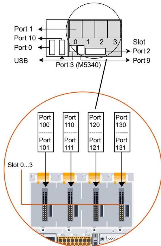
**Slot interface modules made for the following control units**
