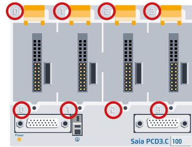
Viewed from the front, each module carrier housing and each module slot has an address field in the lower right corner.
