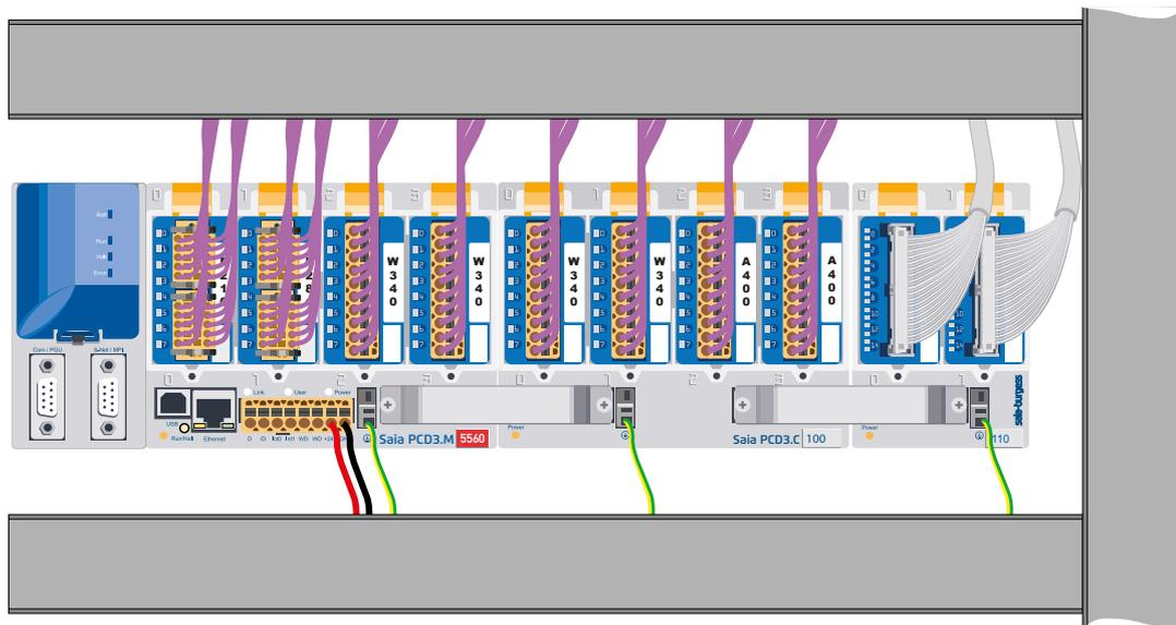
In particular cables to connections on the lower part of the module carrier (supply, grounding) should preferably be wired under the module carriers with a cable duct.
