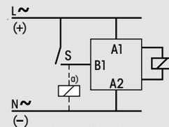
a) A parallel load at B1 is admissible on all CT30 modules.
