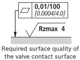
**Item explanations, valve mounting screws and subplates**
