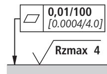
Required surface quality of the valve contact surface
