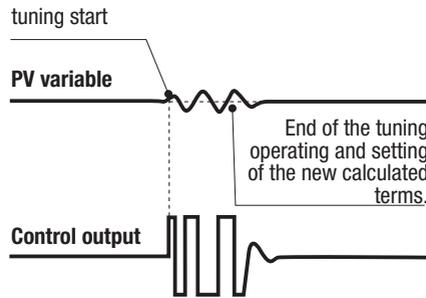
This type is selected when the PV is close to the SP Setpoint. This method has the advantage of a better accuracy in the term calculation with a reasonable speed calculation.
