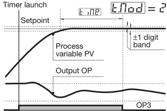
**B - Counting start time inside the band, end with control output forced to zero.**
