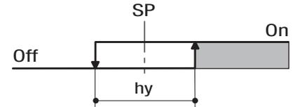
Control or alarm output hysteresis span, set in % of the full scale.
