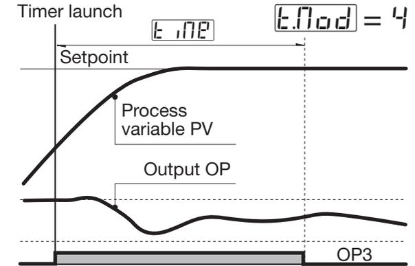
[1] When the Timer is not running the control output is forced to zero, also before the Timer launch
