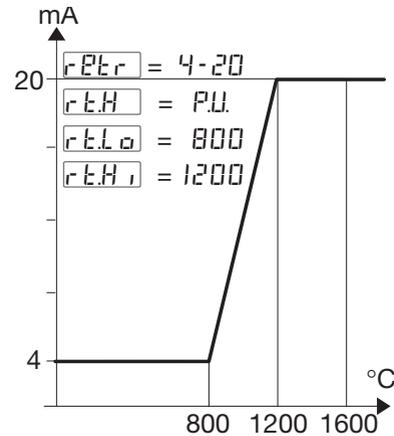
With  $rtlo$  greater than  $rth1$ , it is possible to obtain a reverse scale.
