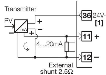
**[1]** Auxiliary power supply for external transmitter 24Vdc  $\pm 20\%$  /30mA max. with no short circuit protection
