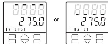
**Note [1]** In case of sensor break, condition, the alarm action is immediate.
