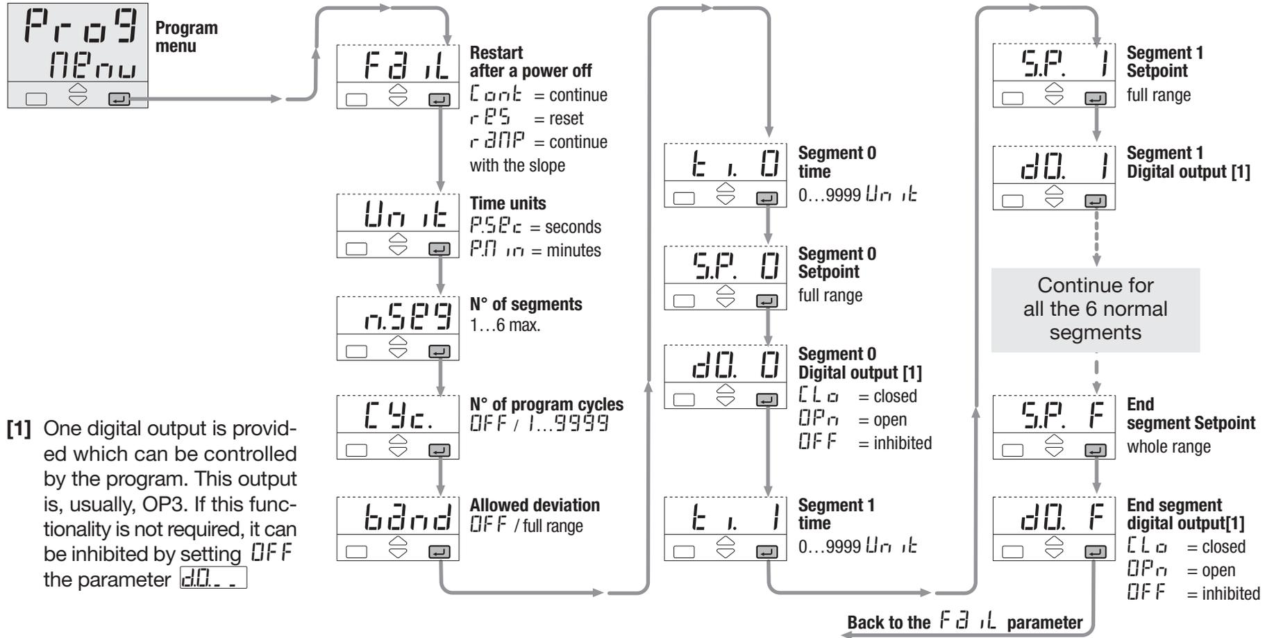
[1] One digital output is provided which can be controlled by the program. This output is, usually, OP3. If this functionality is not required, it can be inhibited by setting OFF the parameter **dO. \_ \_**
