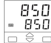
When the Timer is running, the led **RUN** is on.
