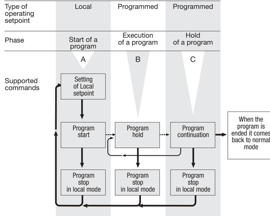
The different phase are displayed in a chained way, just for easing the understanding of the functionality.
