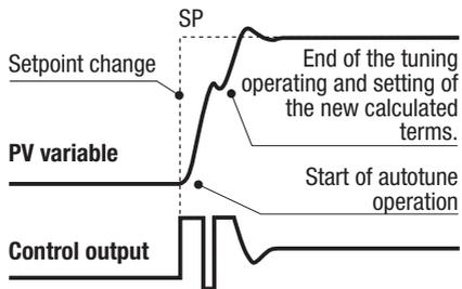
This type is selected when, at the start of the autotune operation, the PV is far from the Setpoint of more than 5% of the span. This method has the big advantage of fast calculation, with a reasonable accuracy in the term calculation.
