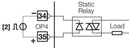
**2.3.5-E DOUBLE ACTION RELAY (TRIAC)/SSR DRIVE CONTROL OUTPUT**
