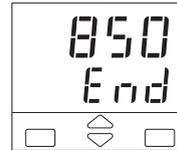
When the Timer ends, the Setpoint display shows alternatively the message `End` and the Setpoint value until a key is pressed.
