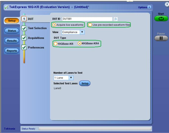
**10GBASE-KR/KR4 Compliance and Debug Solution (Option 10G-KR)** - Automated compliance measurements for IEEE 802.3ap-2007 specifications. This option includes an automated compliance solution and debugging with DPOJET. The automated test setup measures transmitter equalization levels generating 12 results for each tap and 120 results for 1 different measurements in approximately 15 minutes.
