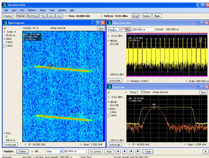
**SignalVu<sup>®</sup> Vector Signal Analysis** – Easily verify wide-bandwidth designs such as wideband radar, high data-rate satellite links, WLAN 802.11, or frequency-hopping radios and characterize wideband spectral events. SignalVu<sup>®</sup> combines the functionality of a vector signal analyzer, a spectrum analyzer, and the powerful triggering capabilities of the MSO/DPO70000 Series – all in a single package.
