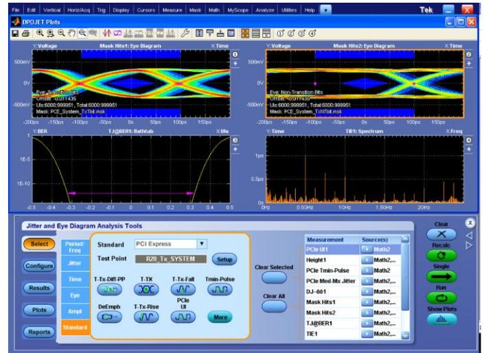
**PCI Express® Transmitter Compliance and Debug (Option PCE3)** – Analyze the performance of your PCI Express® Rev 1.0, 2.0, or 3.0 (draft spec) design with comprehensive test support. Using DPOJET, Option PCE3 enables tests that conform to PCI-SIG standards.
