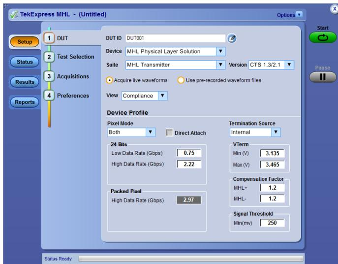
**TekExpress® MHL Advanced Analysis and Compliance Software (Option MHD)** - Provides the most comprehensive solution for MHL 1.0/2.0/1.3/2.1 compliance testing as well as debug and validation of MHL devices against the latest MHL specifications. The application automates Transmitter, Sink and Dongle Electrical tests. Results are presented in a comprehensive HTML format for engineering test documentation
