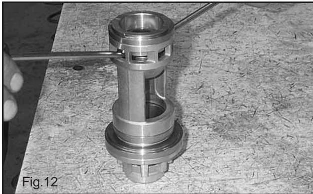
Should excessive scaling inside the fluid end hinder the valve extraction open one of the two lateral inlet port, remove the three plugs 1, Fig.15, insert our special tool p/n 2000.0005.0 (2, Fig.15), or a corresponding one, and push the valve unit out as shown in Fig.15.
