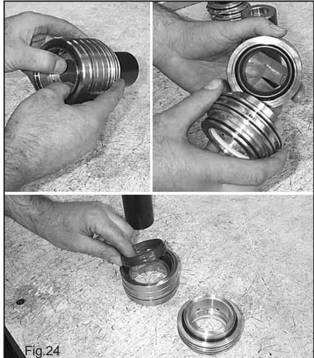
Separate the pumping unit components and check them for wear. Pressure packing replacements is carried out by hands without need of special tools (Fig.24)
