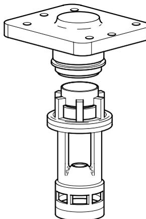
Valve components of each valve unit are pressed together in one single block and therefore they can be easily serviced, replaced and installed back in place. Separating the various components of the valve unit is carried out by means of simple tools as shown in Fig. 11, 12, 13 of the next page.
