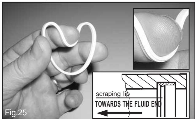
In order to fit the new scraper in place shape it manually as shown in Fig.25.
