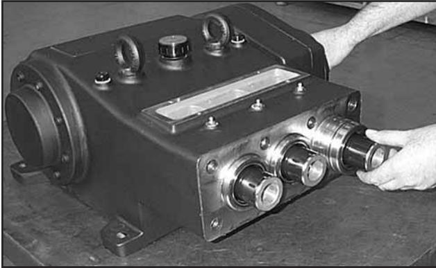
With the tool in place, rotate the crankshaft until the packing support is pushed out together with plungers and cylinders (Fig.21 and Fig.22).
