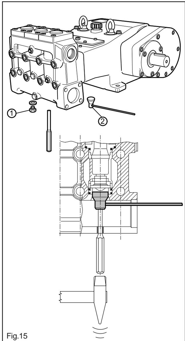
Check the valve components for wear and replace where necessary.
