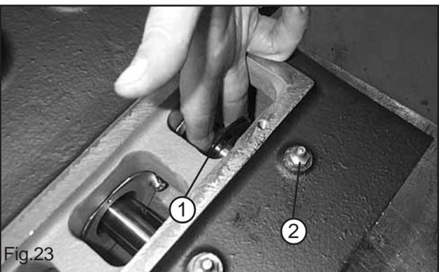
Remove the wipers from the piston guides (1, Fig.23).
