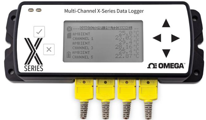
The OM-CP-QUADTCTEMP2000-A2 and OM-CP-OCTTCTEMP2000-A2 are four and eight channel thermocouple data loggers with an LCD screen. The device features on-screen minimum, maximum and average statistics, as well as a user configurable screen that allows for any combination of channels to be displayed. The device accepts J, K, T, E, R, S, B and N type thermocouples.
