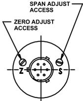
ZERO AND SPAN ADJUSTS ARE PROTECTED BY SEAL SCREWS
