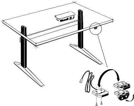
The DPA can be mounted on the desktop so that the keys are either facing upwards or outwards. Alternatively the DPA can be mounted flat under the desktop with the keys facing downwards.
