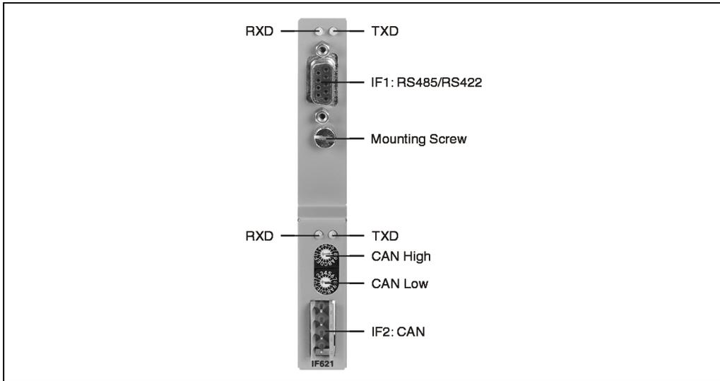
Figure 185: IF621 operational and connection elements
