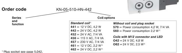
In high humidity environments please use the KN-55-... series with special coils and seals. All dimensions are equal to the KN-05 series. Information about electrical datas see page 4,280,
