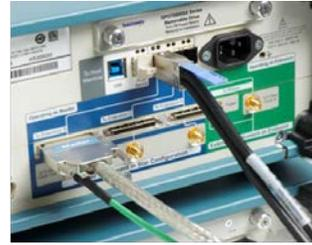
UltraSync connection on instrument with Master role
