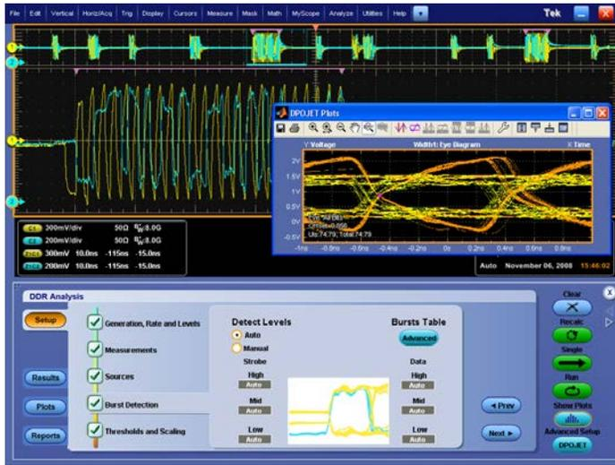
**DDR Memory Bus Analysis (Option DDRA)** – Automatically identifies DDR1, LPDDR, LPDDR2, LPDDR3, DDR2, DDR3, DDR4, and GDDR3 Reads and Writes and makes JEDEC conformance measurements with pass/fail results on all edges in every Read and Write burst. DDRA provides capabilities for measurements of clock, address, and control signals. In addition to enabling conformance testing DDRA with DPOJET is the fastest way to debug complex memory signaling issues.
