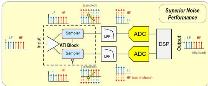
With two copies of the entire signal energy digitized, the signal spectra are "unfolded" using a DSP equivalent of the sampling process and combined to reproduce the input signal. Because two copies of the signal are being combined the process effectively averages them together, reducing random noise. Phase-inversion introduced by the sampling process causes intermediate frequency components to directly cancel one another, simplifying reconstruction and calibration.
