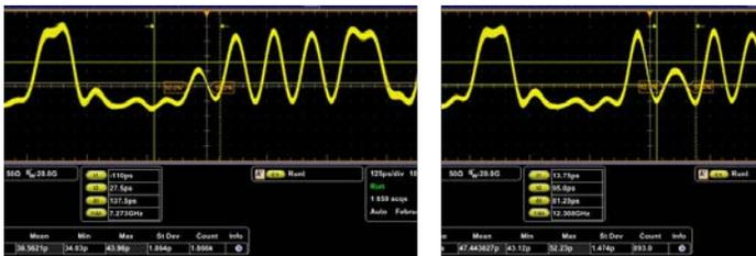
In the next figure, pulse width discrimination is used to isolate pulses >40 ps and <60 ps wide, showing reliable capture of 50 ps pulses within a 20 Gbps PRBS11 sequence.
