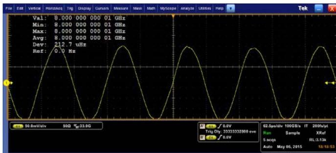
This feature provides the ability to make highly accurate clock stability measurements. In the screen capture shown, a deviation of 212 μHz of source wander is measured on an 8 GHz precision source. In this figure, the signal generator was set to 8.00000000001 GHz, and the scope measured precisely that amount.
