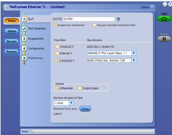
**Ethernet Transmitter Test Application (Option XGBT2 and NBASET)** - Automates 10GBASE-T, NBASE-T, and IEEE802.3bz (2.5G/5G) physical medium attachment (PMA) and physical-layer (PHY) electrical testing to provide a fast and accurate way of testing your Ethernet designs.
