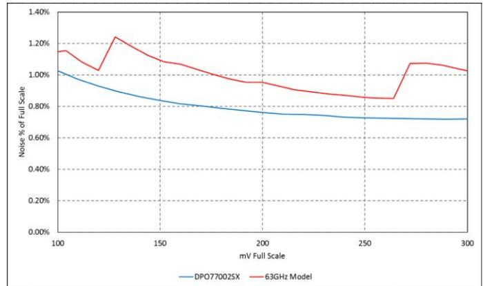
DPO77002SX vs. other vendor's 63 GHz model: Baseline noise % of FS vs. mV<sub>FS</sub> setting, with trace centered, at 60 GHz BW, maximum sample rate setting (200 GS/s or 160 GS/s)
