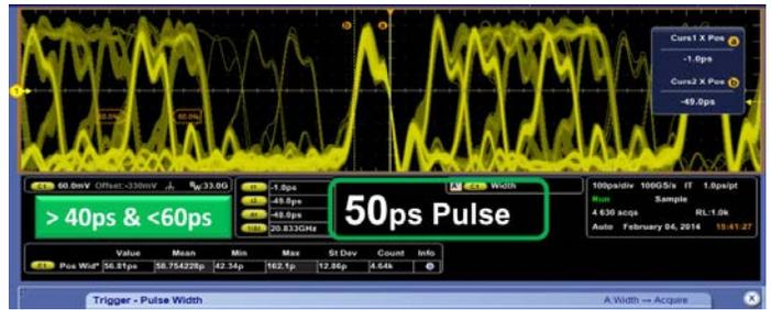
DPO7000SX includes a unique Envelope trigger mode that enables direct triggering on the envelope of a modulated carrier. Edge, Width and Timeout trigger types can be applied to a detected envelope to provide stable trigger on modulated bursts or discriminate bursts of a specific width. Carrier frequency can range from 500 MHz to 20 GHz to address a broad range of applications. The figure illustrates triggering on burst of specific width.
