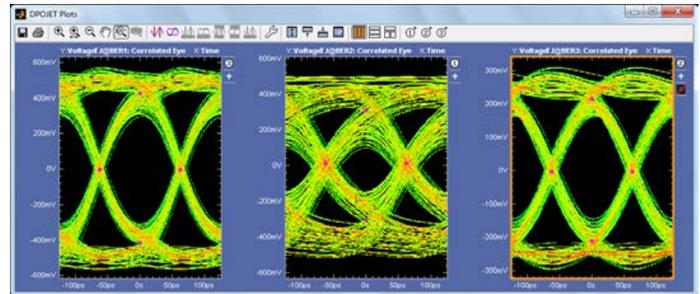
**Custom filters** – Create your own filters or use the filters provided standard with the DPO7000SX Series to enhance your ability to isolate or remove a component of your signal (noise or specific harmonics of the signal). These customizable FIR filters can be used to implement signal-processing techniques, such as removing signal pre-emphasis or minimizing the effects of fixtures and cables connected to the device under test.
