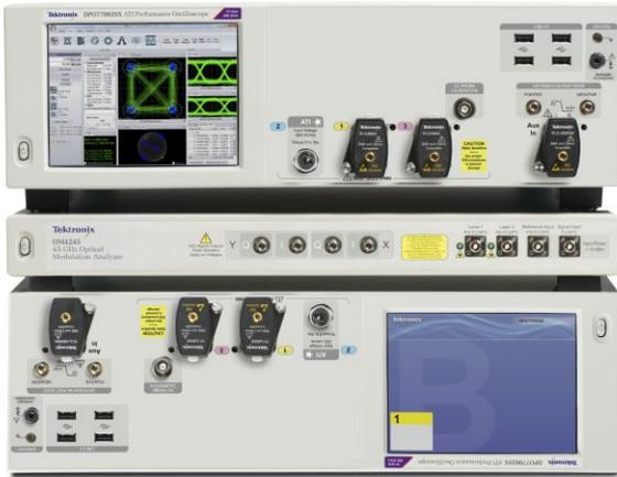
DPO70000SX units may even be operated inverted if desired, to shorten OMA receiver connection distance as shown.
