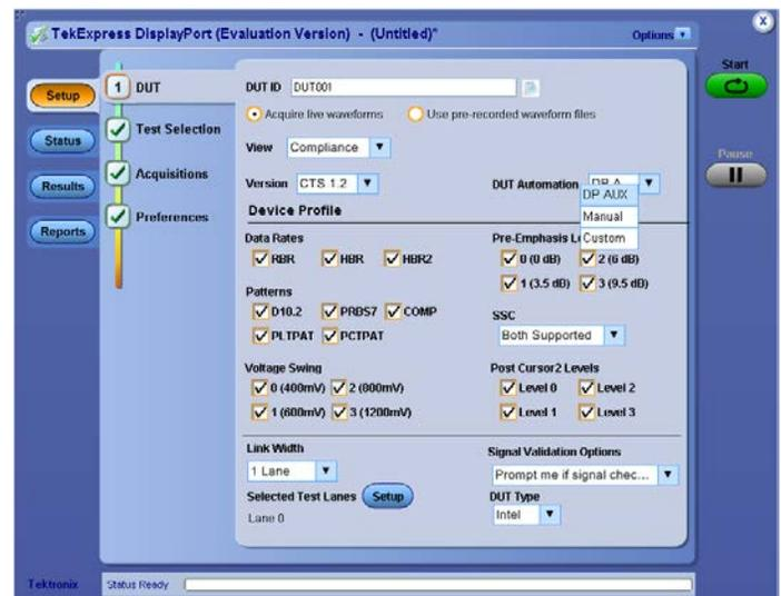
**DisplayPort Compliance Test Solution (Option DP12)** – Supports DisplayPort Compliance Test Standard (CTS) source test with four-line simultaneous testing using the Tektronix® P7300SMA Series probes and DisplayPort software. Detailed test reports with waveform plots, pass/fail results, and margin analysis are included.
