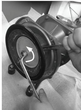
Pic. 4: Diaphragm disassembly
