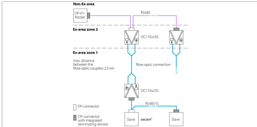
The optocoupler OC11Ex/3G.2 converts the PROFIBUS-DP signals into optical signals. The bus signals can therefore be transmitted from the safe area to the Ex area over long distances without potential or interference. When using fiber-optic cables, the maximum baud range is 2500 m for OM1 (62.5/125- $\mu$ m) cables and 1500 m for OM2 (50/125- $\mu$ m) cables.
