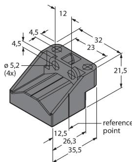
Floating positioning element for linear position sensors LI-Q25L; the nominal distance to the sensor is 1.5 mm; pairing with the linear position sensor at a distance of up to 5 mm or misalignment tolerance of up to 4 mm.
