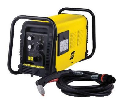
The ESAB Cutmaster 120, weighing only 28 kg and provides 120 amps of cutting power for a 40mm (1-1/2") recommended cut and 55mm (2-1/8") maximum cut. This compact unit, like all other Cutmasters, comes standard with the 1Torch® providing you with the well known comfort and reliability famous throughout the industry. Packages include power source, SL100 1Torch, spare parts kit, air filter/regulator, work cable and clamp and power cable.
