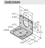
3027162 Mounting bracket, rectangular, stainless steel, for sensors with 30 mm thread, wide holes for accurate alignment
