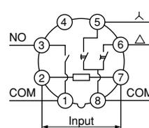
Note: Do not use terminal ③ of the MS4SF-R as a relay terminal because it is connected to terminals ① and ② in the timer.
