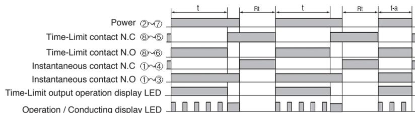
※ We suggest over 100 ms of Min. setting time for D1, E1 output mode because excessive short setting time may cause of malfunction
