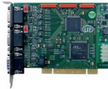
The IF2008 interface card enables the synchronous capture of 4 digital sensor signals series optoNCDT 1420 or others or 2 encoders. In combination with IF2008E a total of 6 digital signals, 2 encoder, 2 analog signals and 8 I/O signals can be acquired synchronously.
