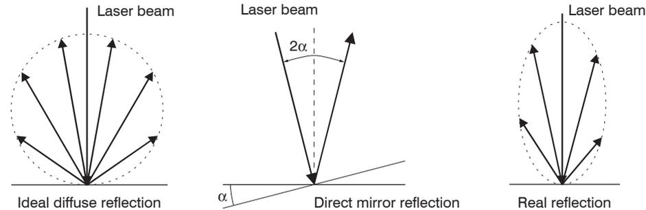
*Fig. 8 Reflection factor of the target surface*
