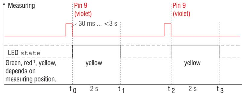
Fig. 35 Flow chart for zeroing, mastering (hardware input)
