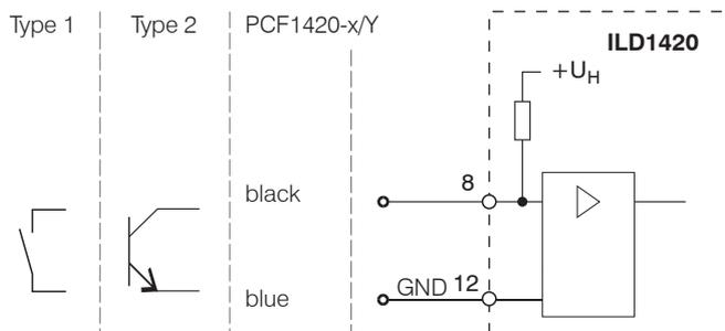
There is no external resistor for current limiting required. Connect Pin 8 with Pin 12 for permanent „Laser on“.
