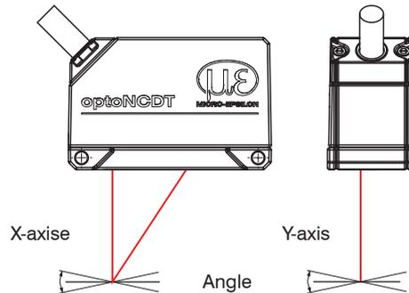
Fig. 9 Measurement errors through tilting with diffuse reflection
