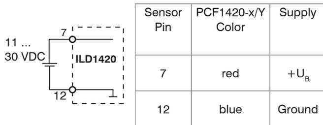
Use the supply voltage for measurement instruments only and not for drive units or similar sources of pulse interference at the same time. MICRO-EPSILON recommends using an optional available power supply unit PS2020 for the sensor.
