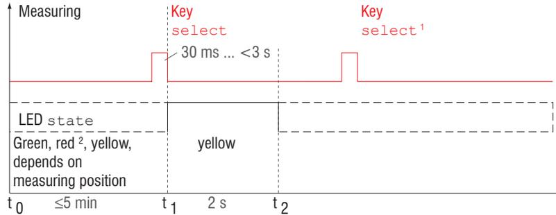
Fig. 33 Flow chart for zeroing, mastering (key select)
