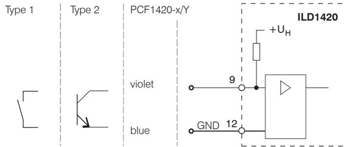
The input is not galvanically isolated. Internal pull up resistance, an open input is noticed as High. Connect the input with GND to trigger the function.
