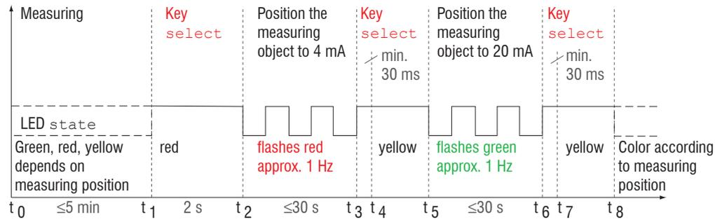
Fig. 40 Flow chart for output scaling
