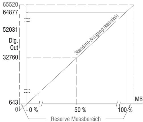
Fig. 37 Digital values without zero setting resp. mastering
