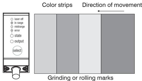
In case of rolled or polished metals that are moved past the sensor the sensor plane must be arranged in the direction of the rolling or grinding marks. The same arrangement must be used for color strips.
