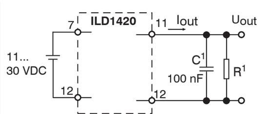
When using a PCF1420-x/U you will get an analog voltage at the output in the range of 1 ... 5 V.
