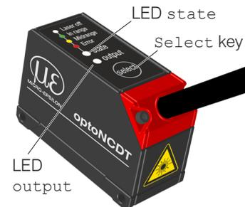
The programmable touch key `select` calls up the functions `Masters` and `Teaching`. By factory default this key is only active for the first 5 minutes after power up. After that it will be automatically locked. The keylock can be programmed via internal websites or ASCII commands.
