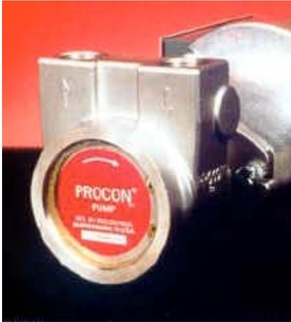
**PROCON pumps** can be mounted to two types of electric motors -- a carbonator style motor (NEMA 48YZ frame) and a C-frame motor (NEMA 56C frame). Pump applications that require a motor of up to 0.75 horsepower, open drip proof construction and single phase power can be close-coupled to NEMA 48YZ frame, carbonator style motors.
