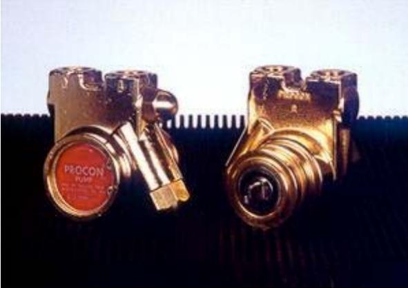
**PROCON Series 1** pumps have the protection of an integral inlet strainer. The standard strainer is a 100 mesh wire screen. It traps particles that can cause serious damage to the pump.
