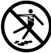
**Do not touch the pump when there is liquid on the floor. Serious injuries can occur if you slip.** Your pump operates with an electric motor. You can be electrocuted if you touch the pump when you are standing in liquid.
