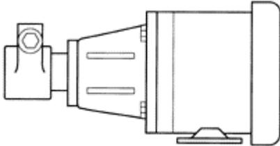
You will need an aluminum "C-face" adapter and shaft coupling to mount your pump to a NEMA 56C frame motor. The adapter and coupling are available from PROCON.
