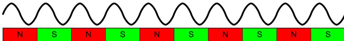
These signals are then interpolated electronically; the resolution of the measuring system is a result of the interpolation rate and the pole pitch.
