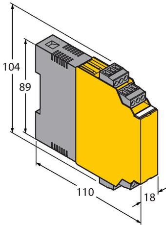
Isolating switching amplifier, 2-channel; 2 relay outputs; input NAMUR signal; selectable ON/OFF mode for wire-break and short-circuit monitoring; adjustable output mode (NO / NC mode); removable terminal blocks; width 18 mm; universal power supply unit
