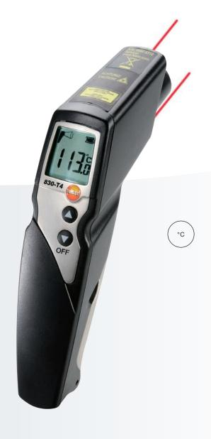
The testo 830 is a universally applicable infrared thermometer for non-contact measurement of surface temperatures in trade and industry. Thanks to a new processor, and therefore better resolution, even more precise measurements are now possible. Temperature can now be recorded to an accuracy of 0.1 °C. Thanks to the min./max. function, the limit values of the last measurement can be displayed and even better monitored.
