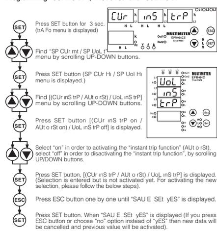
**Programming "SP UoL t":** Using purposes of submenus of "SP UoL t" explained below with details.
