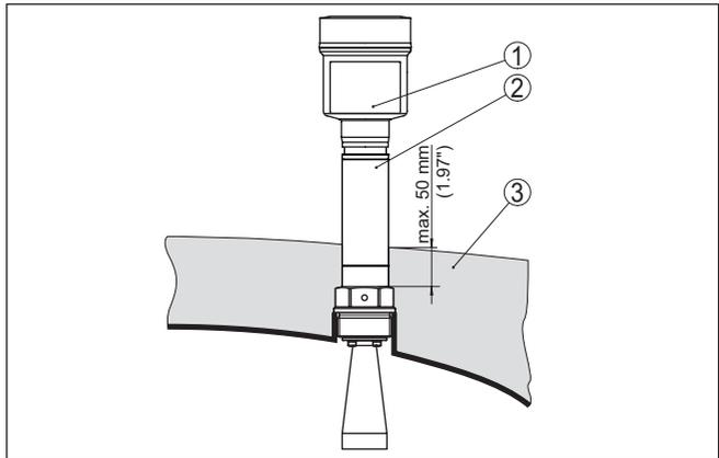
Fig. 16: Mounting the instrument on insulated vessels.
