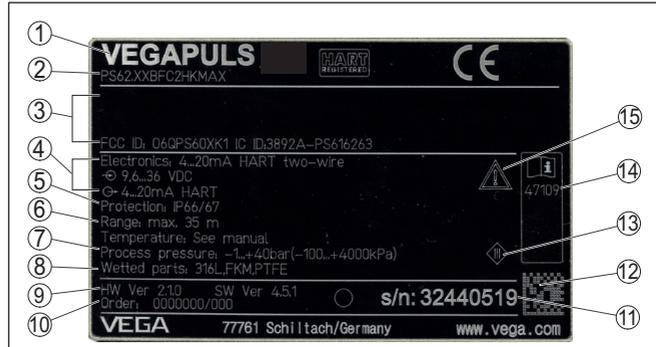
Fig. 1: Layout of the type label (example)
