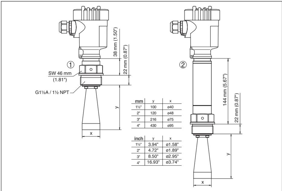
Fig. 63: VEGAPULS 62, horn antenna in threaded version
