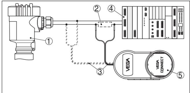
Fig. 39: Connecting the PC via HART to the signal cable
