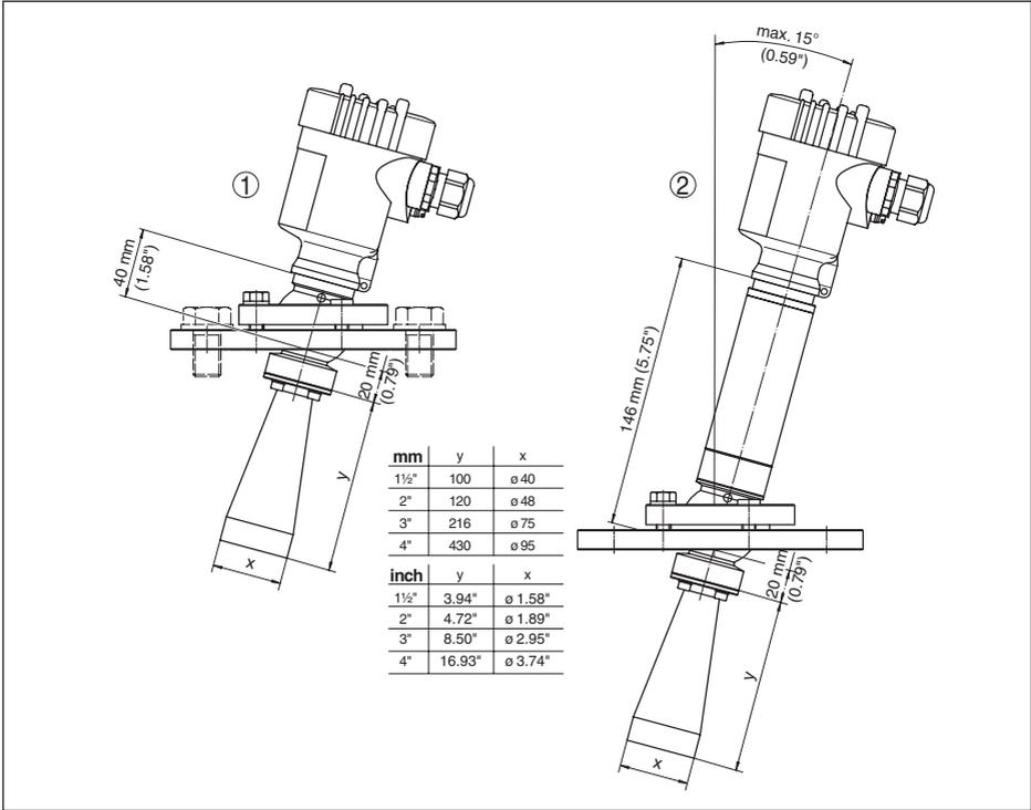
Fig. 67: VEGAPULS 62, horn antenna and swivelling holder
