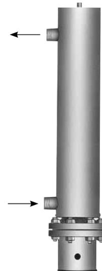
**Vertical Mounting—Gases:** Mount with terminal enclosure and inlet pipe at bottom of tank to minimize terminal box wiring temperatures.
