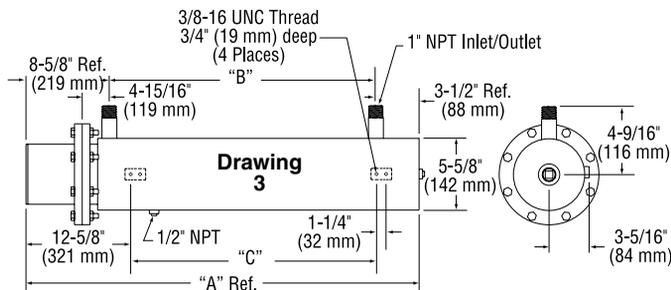
**Note:** Circulation heater mounting lug design and location in the assembly drawings shown are standard. Designs can be modified to fit customer installation. Consult Omega with your requirements.
