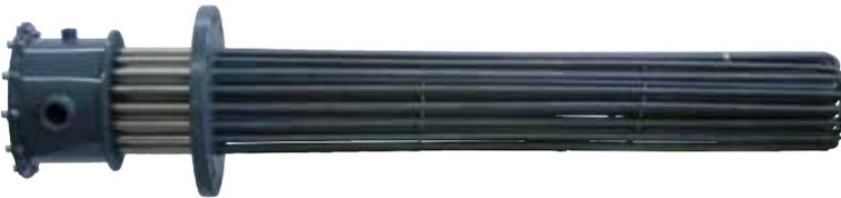
The electrical housing is separated from the flange by an air gap (six-inch standard) to lower the ambient temperature of the electrical wiring. This option is used on flanged immersion heaters where the flange temperature exceeds 250°C (482°F).
