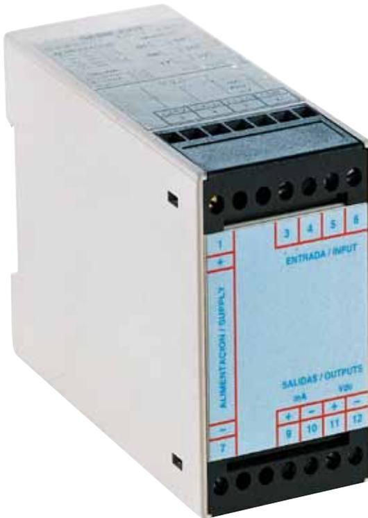
The CCT series of ac and dc input signal conditioners accept analog signals and provide conditioned, isolated analog outputs of 0 to 10 V or 0/4 to 20 mA. The CCT-01 accepts dc voltages, the CCT-08 accepts ac voltages, while the CCT-04 and CCT-32 accept ac and
