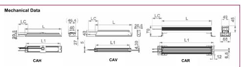
CAH shown with CLIP-ON external thermo watch TW External thermo watch is possible for CAH and CAV. Internal thermo watch (TW) for all types require 25 mm extra length of the housing.
