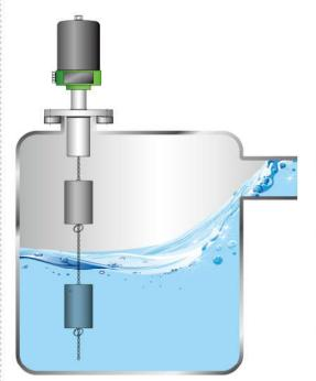
Product should be installed at the place far from inlet in order to avoid the malfunction.
