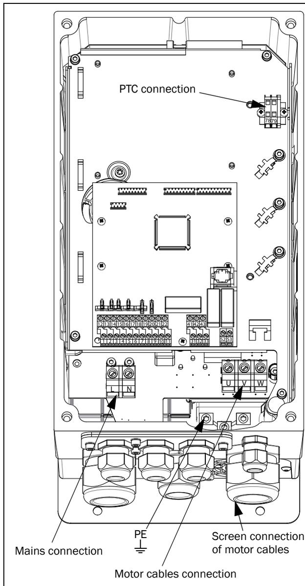
Fig. 7 Mains, motor and PTC connections to Control unit.
