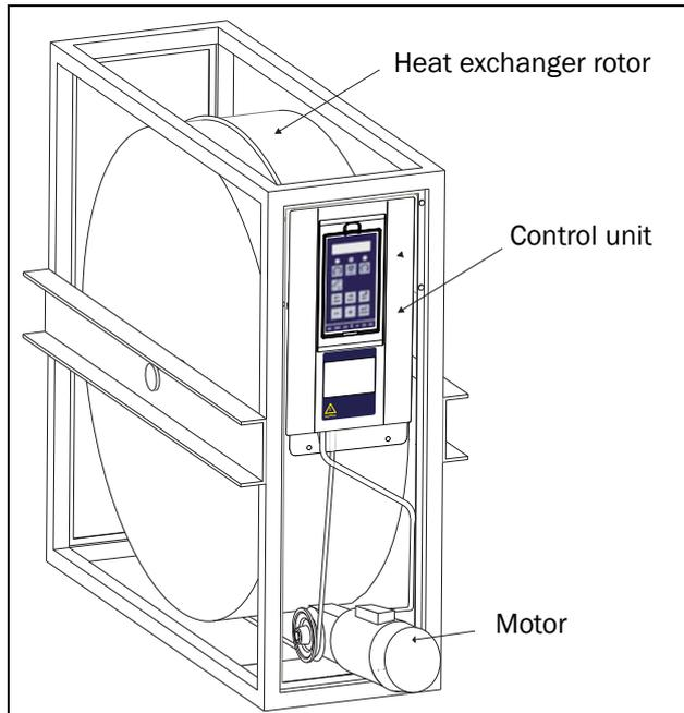
Fig. 4 Emotron motor and Control unit for rotary heat exchangers
