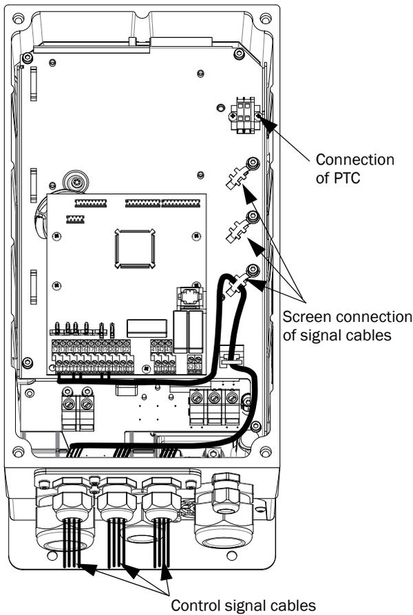
Fig. 12 Connecting the control signals and PTC
