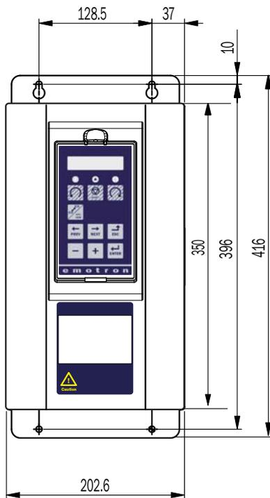
Fig. 36 Dimensions, control unit
