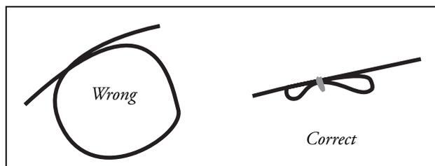
Fig. 1 Excess motor cable should be arranged such that the area enclosed is as small as possible
