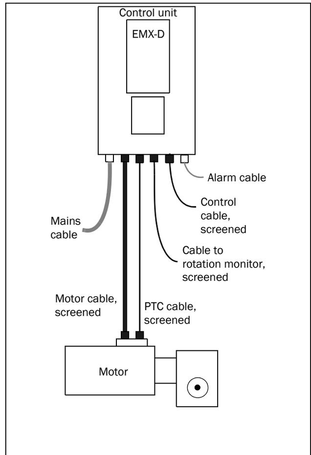
Fig. 9 EMC-adapted installation of EMX-D
