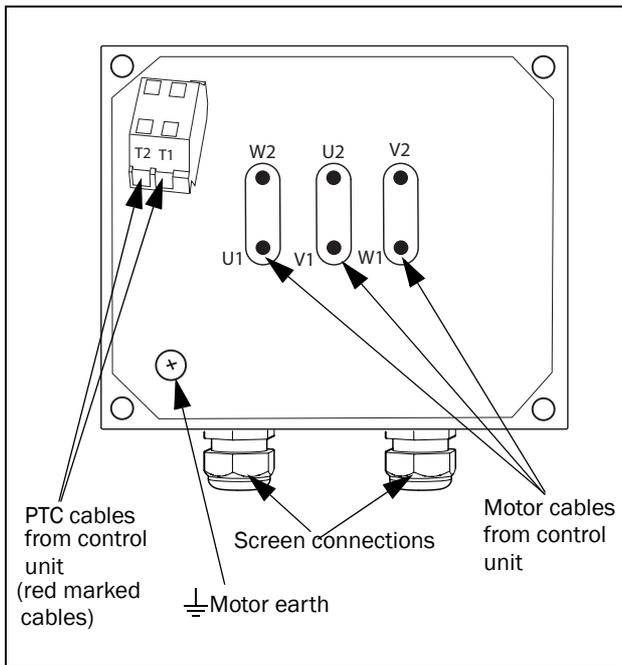
Fig. 8 Motor and PTC cables connection to motor, 3- phases and protective earth plus PTC cables, all screened.
