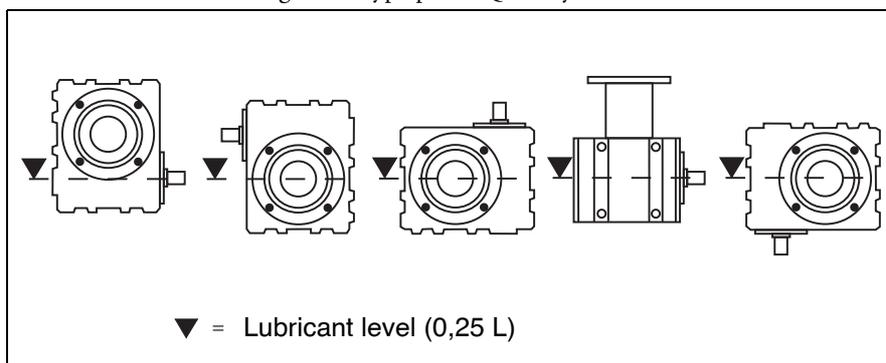
Fig. 1 Recommended oil level in the gearbox depending on shaft position.
