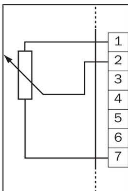
Fig. 13  $10 \text{ k}\Omega$  potentiometer
