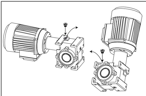
Fig. 2 Remove the plug in highest position and replace with the ventilation plug.
