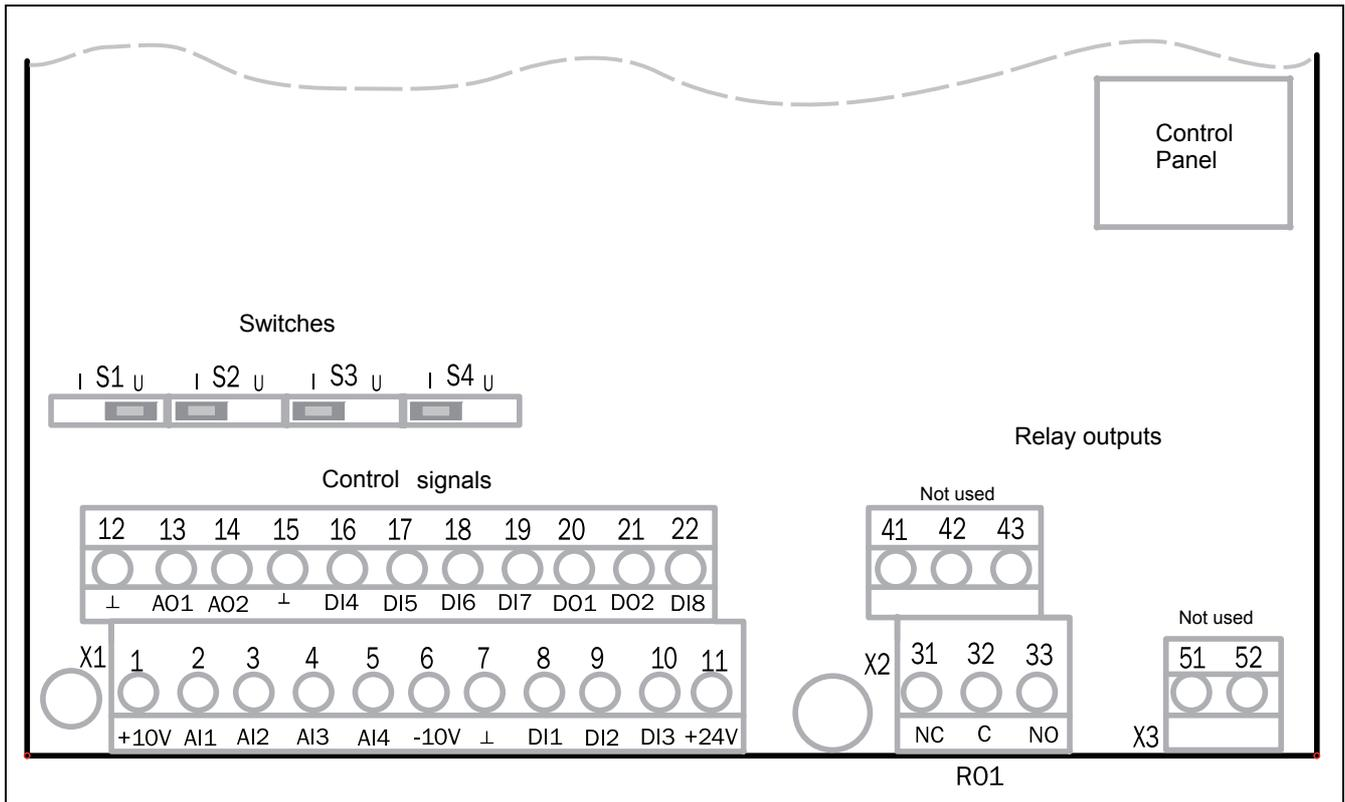
Fig. 10 Control board layout
