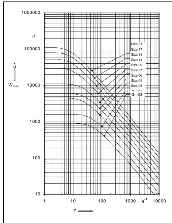
Fig. 24/1: Max. switching work  $W_{max}$  per switching operation as a function of the number of switching operations per hour  $Z$  (values based on  $n=1000$  rpm)
