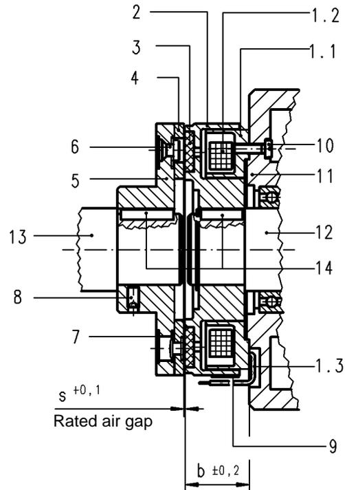
Fig. 5/1: Electromagnetic single-face clutch 86 011..E00 with flange hub (5)
