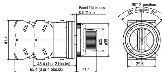
Terminal Screws: M3.5 Terminal cover: integrated
