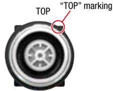
② On non-illuminated models, install the color insert in the middle of operator. The color insert also serves to retain the operator.
