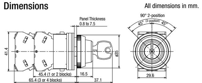
Terminal Screws: M3.5 Terminal cover: integrated
