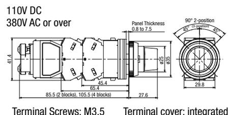
Terminal Screws: M3.5 Terminal cover: integrated
