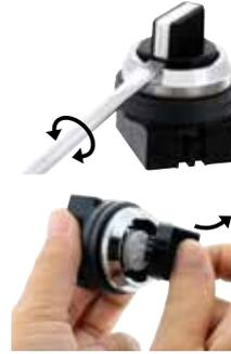
① Insert a flat screwdriver into the recess under the color insert. Turn the screwdriver to push out the insert from the operator.
