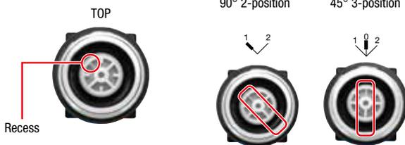
The non-illuminated operators can be installed in positions other than the standard position shown above.
