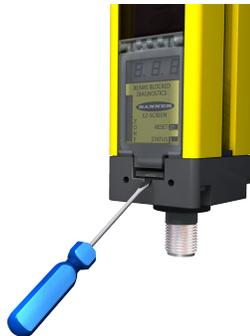
3. Pivot the screwdriver against the bevel until the access cover pops open.
