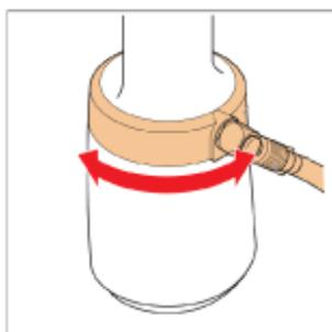
The 360° revolvable air supply unit can be turned in any position so that the hose does not obstruct your work space. Thus providing a comfortable and safe work environment.
